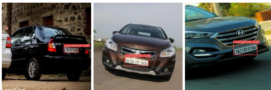
Figure 6: Above images are the results obtained when Phase I i.e. detection phase is performed on car images with different conditions. In first image sideways view of license plate of car is present, in second image normal front view of license plate is present and in third image low resolution vehicle picture is present. Although these conditions are different from each other and can be caused in real-time, our detection model accurately detects license plate with high confidence.
