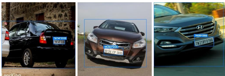
Figure 8: Above images are the results obtained when Phase II i.e. recognition phase is performed on car images with different conditions. In first image sideways view of license plate of car is present, in second image normal front view of license plate is present and in third image low resolution vehicle picture is present. After successful detection of these license plates, our recognition model accurately recognises license plate characters.
